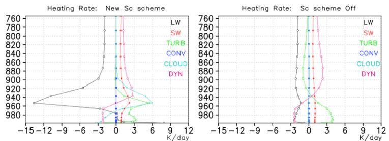
**Fig. 3:** Heating-rate profiles for each physical process for the area off California shown in Fig. 1a and 1c for July. Heating rate for longwave (black) and shortwave (red) radiation, turbulence (green), convection (blue), cloud (light blue), and dynamic (pink) processes with the new stratocumulus scheme (left) and without a scheme (right) for the period 2005–2014 are shown. The vertical axis shows pressure (hPa).
