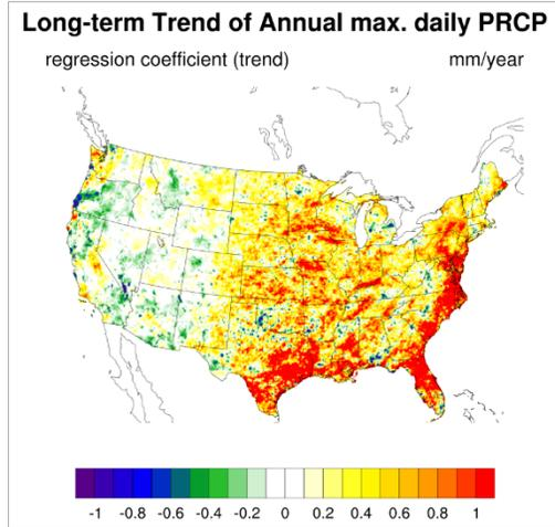
Figure 1. Long-term trend of annual maximum precipitation intensity based on 37 year of data from 1981 to 2017. The data is an observation-based gridded dataset on spatial resolution of 4km, called PRISM.
