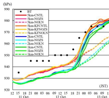
Figure 2. Time series of RMSC Tokyo best track (BT) central pressure and simulated central pressures.
