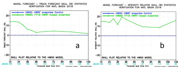
FIG. 1 Comparison of (a) track and (b) intensity forecast skill between HWRF-EPS (HWMN, green) and its deterministic version (blue).
