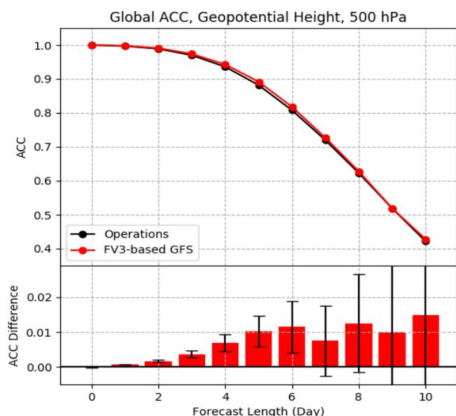
Figure 1: Global time-averaged 500 hPa anomaly correlation coefficients (ACC) as a function of forecast lead time (top) for the operational GFS (black) and the FV3-based GFS real-time parallel (red) with forecasts initialized at 00 UTC for January 27 - April 24, 2019. The bottom panel shows the difference between the FV3-based GFS and the operational GFS for the same timeframe. The error bars represent 95% confidence threshold as derived from a student t-test.
