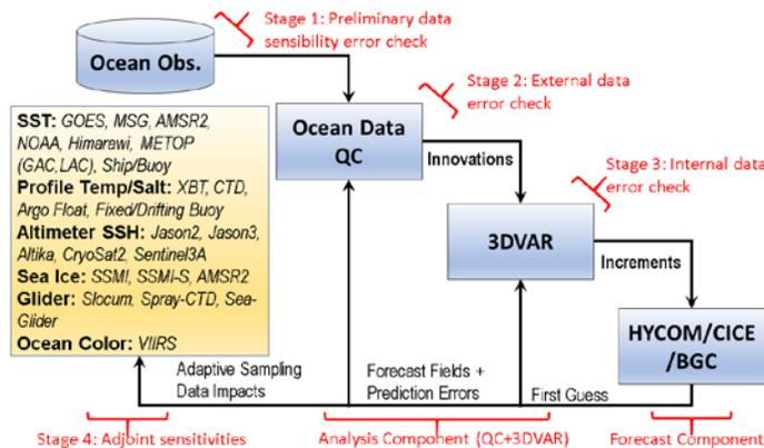
**Figure 1.** A schematic diagram of ocean data assimilation in the NCODA system. Note that oceanographic and satellite data products are available as of 2018.
