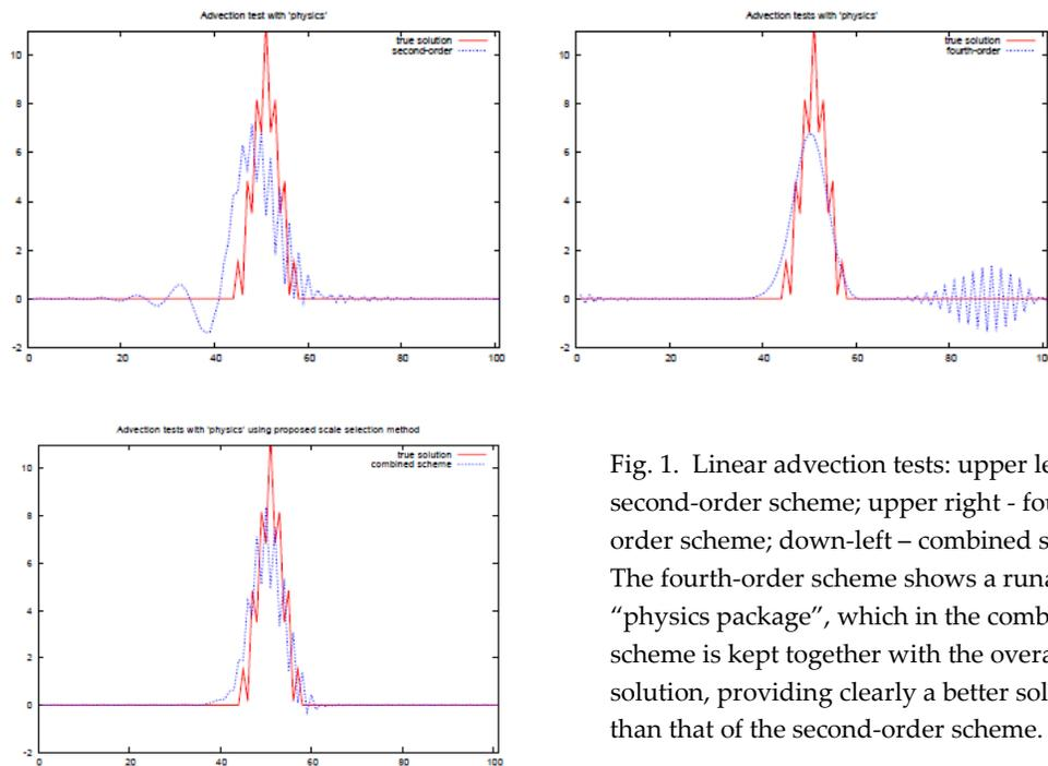
Fig. 1. Linear advection tests: upper left - second-order scheme; upper right - fourth-order scheme; down-left – combined scheme. The fourth-order scheme shows a runaway “physics package”, which in the combined scheme is kept together with the overall solution, providing clearly a better solution than that of the second-order scheme.
