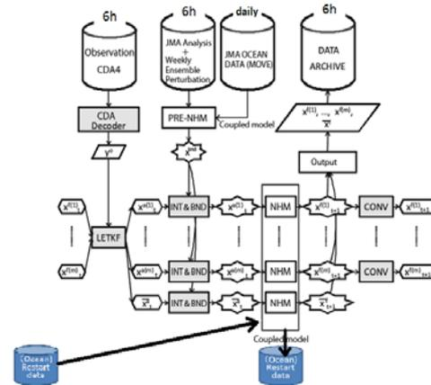
Figure 1 Schematic diagram of NHM-LETKF coupled with the atmosphere-wave-ocean model in the prediction part with oceanic reanalysis data.
