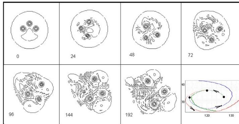
Figure 4. Dynamics of three vortices and their trajectories of movement, derived with the model research. The integration time (in hours) is given in the left bottom corner.
