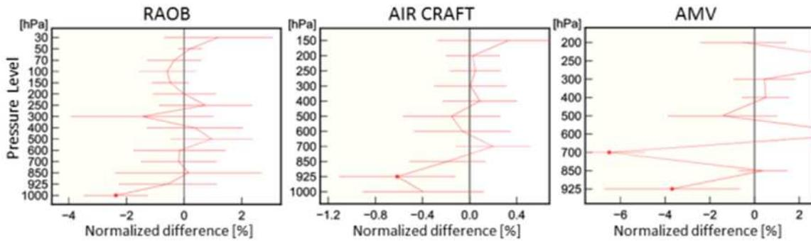
Figure 1: Normalized difference of STDV for the first-guess departure of wind speed ( $(STDV_{TEST} - STDV_{CNTL}) / STDV_{CNTL}$ ) with regard to rawinsonde (RAOB) observation, aircraft observation and AMVs in the January 2014 experiment. Negative values represent improvement. The horizontal axis indicates normalized STDV difference and the vertical axis indicates vertical levels. The error bars represent a 95% confidence interval, and the red dots represent statistically significant values.
