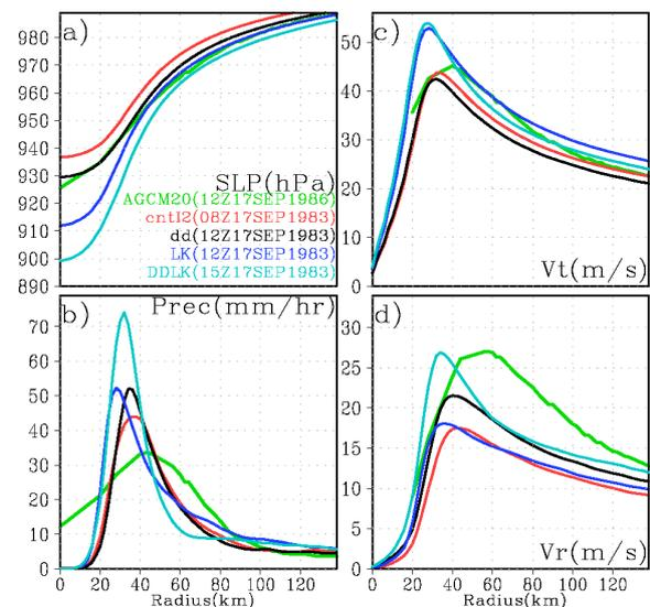
Figure 3 Radial profiles of 24-hourly mean azimuthally averaged a) sea level pressure, b) precipitation, c) tangential wind and d) radial wind speed at a height of 10 m during the rapid intensification phase. AGCM20: green, CNTL2: red, 2dd: black, 2LK: blue, 2ddLK: cyan.
