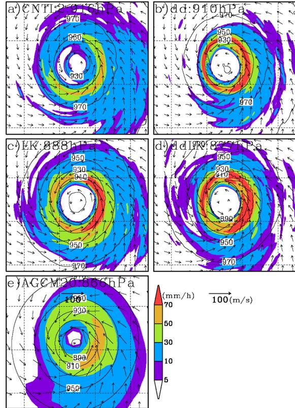
Figure 2 Horizontal distributions of hourly precipitation amounts in the 1 h preceding the most intense phase of the TC: a) CNTL2, b) 2dd, c) 2LK, d) 2ddLK and e) AGCM20. The MCP is indicated in each panel. Arrows indicate 10 m level winds.
