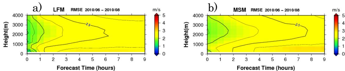
Fig. 4: RMSE of wind speed against WINDAS: (a) LFM; (b) MSM
