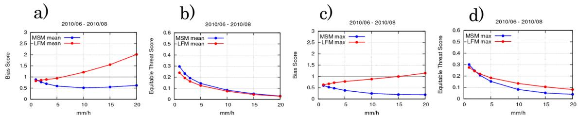
Fig. 2: (a) Bias scores for hourly rainfall amounts according to the LFM (red line) and the MSM (blue line) against the threshold of rain intensity (averaged for each 20-km square mesh on land and over the sea in coastal areas); (b) as per (a), but for equitable threat score (ETS); (c) as per (a), but for the maximum in each 20-km square mesh; (d) as per (c), but for ETS
