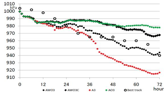
Fig. 1 Time series of Hai-Tang's best-track central pressure every six hours and hourly predicted central pressures in A3, AO3, AWO3, and AWO3C.
