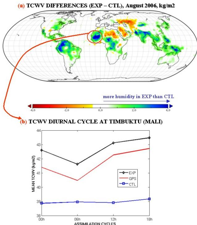
Figure 1 : (a) Mean TCWV analysis differences (experiment minus control) during August 2006. Negative (positive) values indicate that the control assimilation is more moist (dry) than the experiment. (b) Diurnal cycle of TCWV near TOMBOUKTOU estimated using GPS measurements and using analyses from CTL and from EXP assimilation experiments. Statistics are for 45 days (from 01/08/2006 to 14/09/2006)
