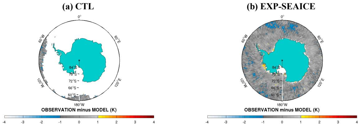
Figure 2 : Departures from First guess for assimilated AMSU-B channel 5 ( $183.31 \pm 7.0$  GHz) observations from (a) a CTL experiment and from (b) an experiment making use of a new sea ice emissivity model. Statistics are for 2 weeks (from 25/12/2008 to 06/01/2009)
