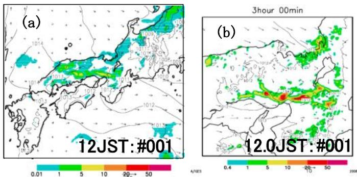
Fig. 5. Rainfall distribution at 12 JST (03 UTC) reproduced by the downscale experiments using the NHM with the grid intervals of 5km and 1.6 km.
