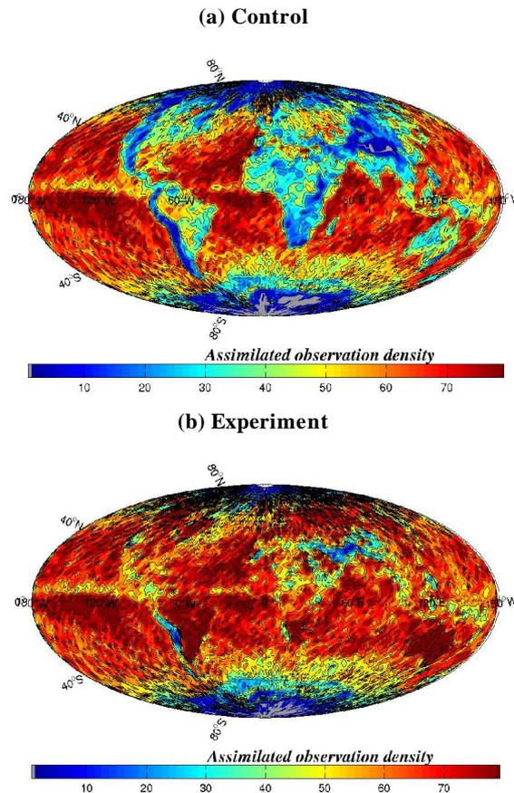
Figure 1: Density of assimilated observations (number of assimilated observations over a  $2^\circ \times 2^\circ$  grid) from AMSU-A channel 7 and over August 2006. Results are given for (a) the control and for (b) an experiment that uses dynamically varying emissivities derived at AMSU-A channel 3.
