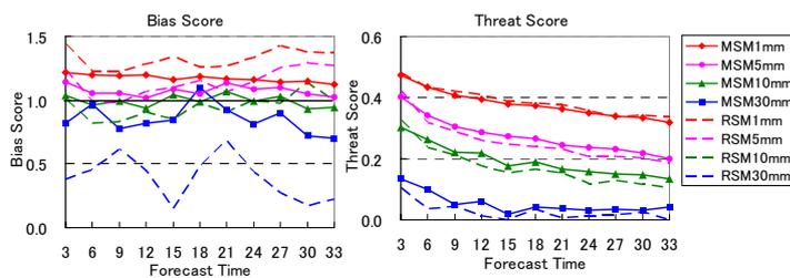
Fig.1. Time sequences of bias and threat scores by MSM0705 and RSM. "MSM1mm" denotes the score of MSM0705 for 1mm/3h.
