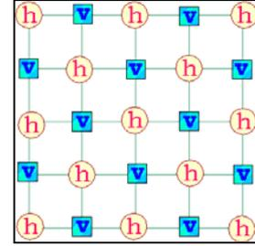
**Figure 1. Grid spacing of height and velocity points**
