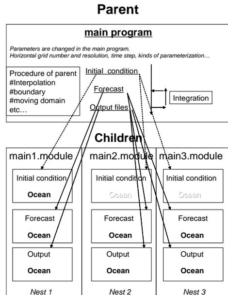
Figure 1. The system of MRI interactive multiply-nested movable mesh tropical cyclone model.
