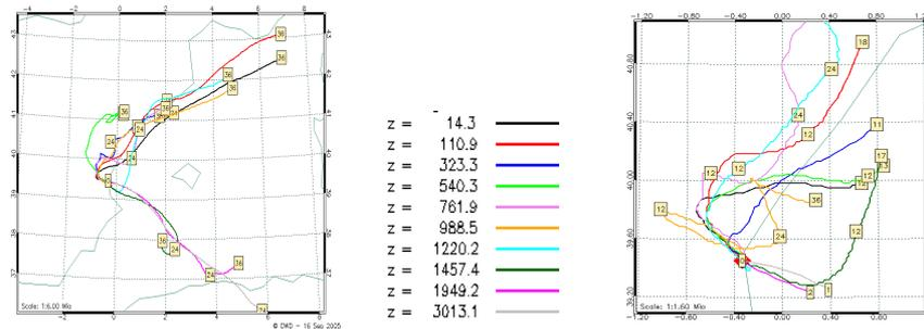
Fig. 1: LM trajectories starting at identical station at height  $z$  [m] on Valencia coast, Spain, 28 Sep 1999, 11UTC. Left: 7km, right: 1.1km resol. with improved local re-circulation leading to increased pollution levels.
