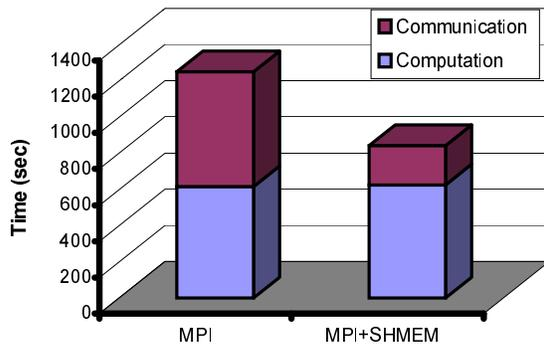
Fig. 2. Comparison of communication and computation costs for T339L31 based on MPI only and on MPI + SHMEM (32 PEs).
