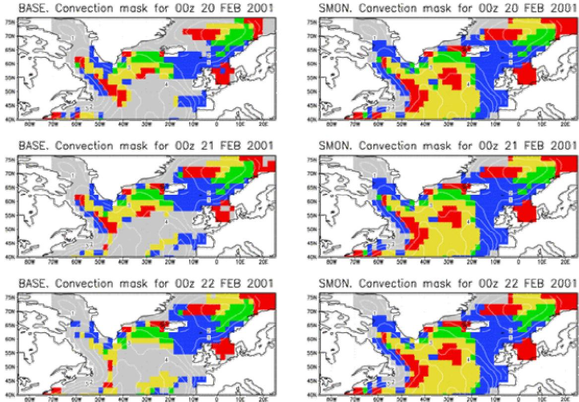
Fig. 1. Horizontal structure of convection events in the North Atlantic during February, 20–22, 2001 in runs **BASE** with 6-hr atmospheric forcing (left panels) and **SMON** with monthly smoothed forcing (right panels).
