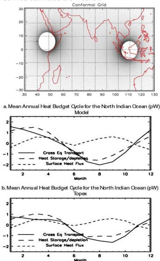
Figure 1. The global varying resolution grid used in the MICOM Indian Ocean Model. Only the Indian Ocean portion is shown. The poles are placed over land and thus avoiding the singularity problem. The resolution varies from  $0.2^\circ - 0.5^\circ$  in the northern Indian Ocean and  $0.5^\circ - 1^\circ$  in nearby basins.
