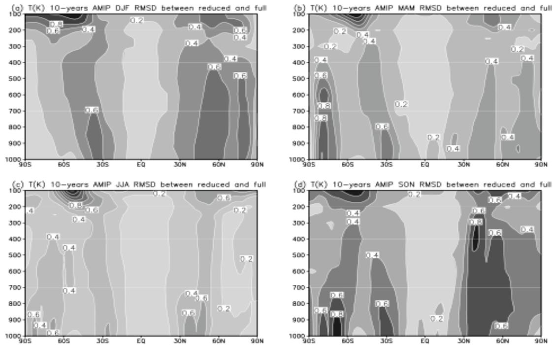
Fig 2. Root Mean Square Difference (RMSD) of 10-year zonal seasonal-mean temperature between reduced and full spherical transforms, plotted for (a) winter, (b) spring, (c) summer, and (d) fall, with contour interval of 0.2 K.
